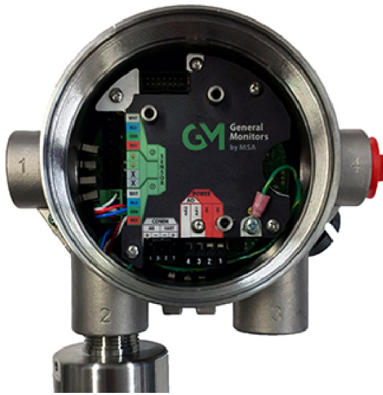
Fig. 13 Connecting Sensor to the Stack and Grounding Terminal
