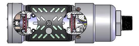
Figure 8: IR400 Optical Window Locations
