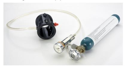
The portable purge calibrator is a compact, accurate and safe system containing a non-explosive gas concentration. The lecture bottle is filled with a standard 50% LEL mixture of gas/air. Using a known gas/air mixture reduces the likelihood of error in field calibration.
