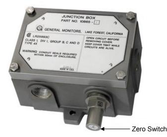
**Zero the Unit**. Apply the General Monitors magnet that was included with the unit to the Zero Switch / LED for approximately three seconds. The LED in the switch will light to show proper placement.
