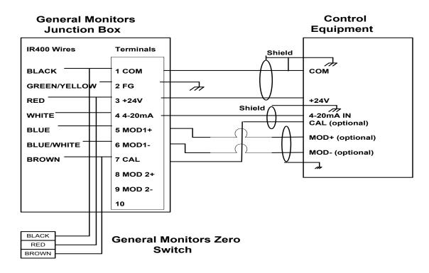
Figure 2: Wiring Diagram from IR400 to Control Equipment
