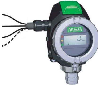
Fig. 5 3-wire/4-wire connection - PrimaX P
