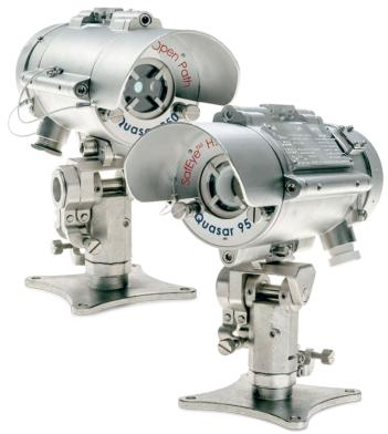
The Quasar 950 is part of the innovative SafEye Quasar open path gas detectors series, provides UV technology continuous monitoring for toxic hydrogen sulfide (H2S) gas at very low concentrations, up to 95% obscuration, featuring advanced long range detection at up to 200ft (60m), high-speed response in under  $\square$ 10 sec.
