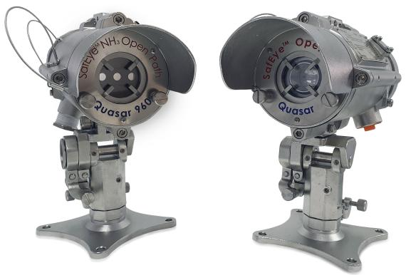
The Quasar 960 is part of the innovative SafEye Quasar open path gas detectors series, provides UV technology continuous monitoring for toxic ammonia (NH3) gas at very low concentrations, up to 95% obscuration, featuring advanced long range detection at up to 200ft (60m), high-speed response in under  $\Box$  10 sec.
