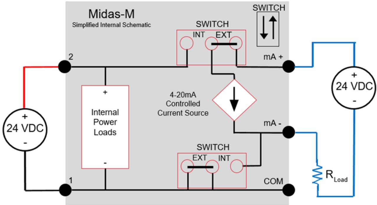
Generic example Midas-M 3-wire Sinking output
