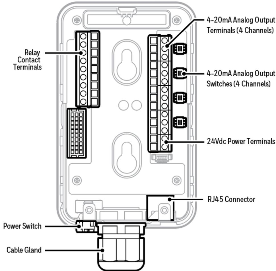
The terminals used are suitable for conductors of 24 to 14 AWG (0.5 to 1.8mm Dia.). We recommend using the 16 AWG (1.5 mm Dia.) conductors.
