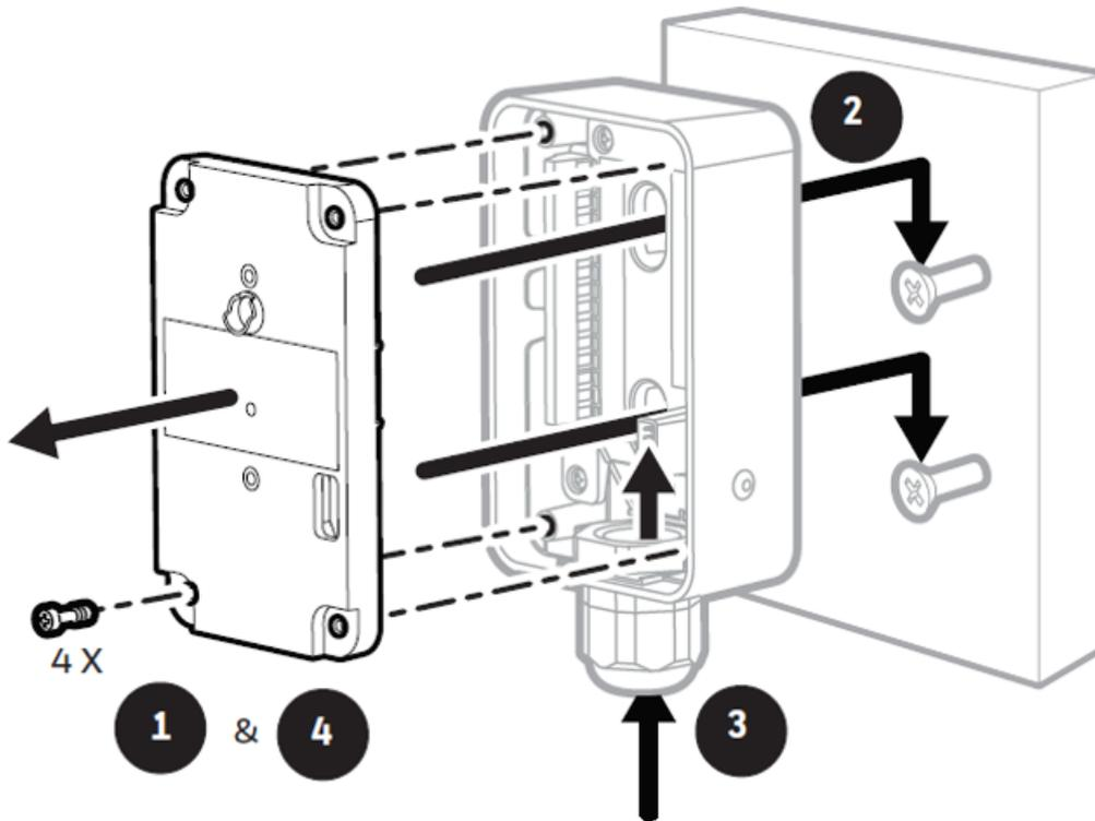
5. Push the mounting bracket assembly horizontally and engage the Relay Module connector.
