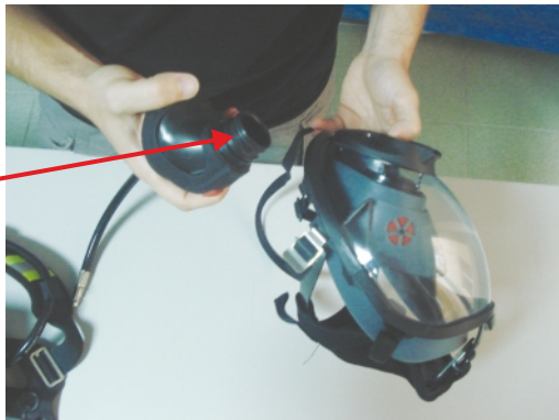
Figure 11 Visual checking of second stage reducer and face mask
