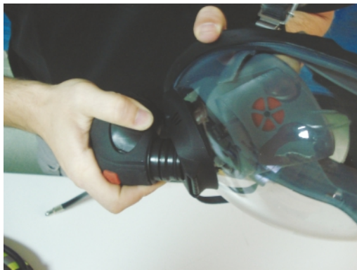
Figure 12 Assembly of the second stage regulator with the face piece
