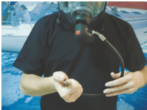
Figure 13 Face piece leak tightness test
