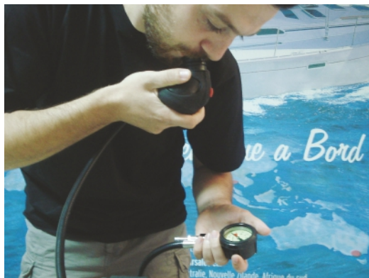
Figure 9 "ON DEMAND" valve operability check
