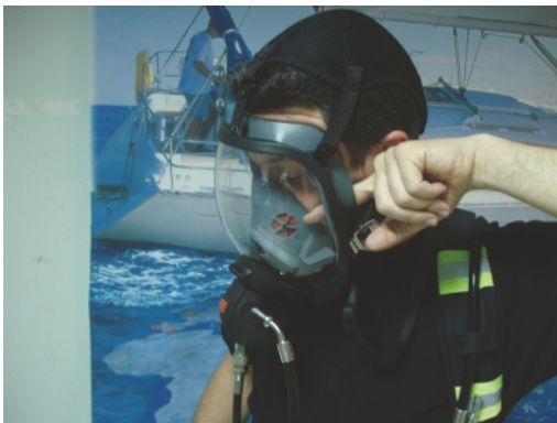
Figure 21 Face Seal Check Method
