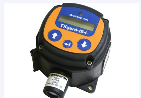
TXgard-IS+ is an Intrinsically Safe (I.S.), 2-wire, toxic and oxygen gas detector with local LCD display. A wide choice of sensors is available for use in a variety of applications. TXgard-IS+ is ATEX and IECEx certified for use in Zone 0,1 or 2 hazardous areas.
