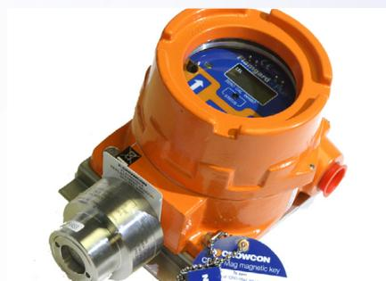
Flamgard Plus is a Flameproof (Ex d), ATEX and IECEx certified flammable gas detector, which uses poison-resistant pellistors to detect explosive levels of hydrocarbons, hydrogen and other flammable gases and vapours, including aviation fuel and leaded petrol vapours.
