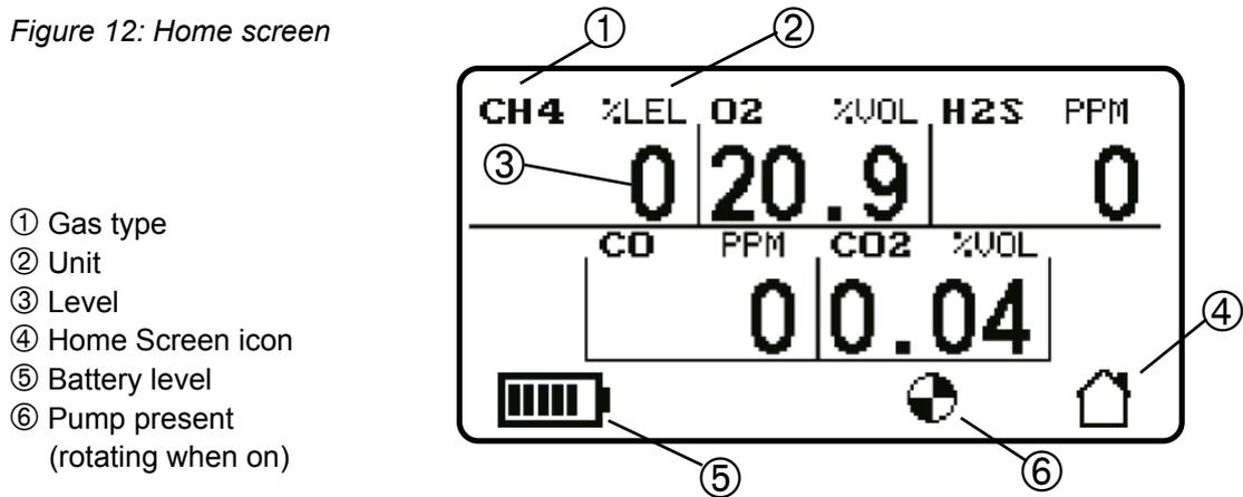
In 'clean air', CO<sub>2</sub> and Oxygen levels are typically 0.04% and 20.9% respectively. In zero mode, these gases will actually run an 'offset' zero.
