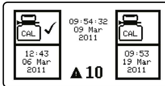
If the calibration due lockout feature has been enabled the lockout icon
