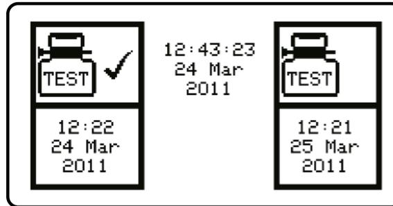
The next screen indicates when the Gas-Pro was last calibrated. It also indicates when the next calibration is due with a warning symbol
