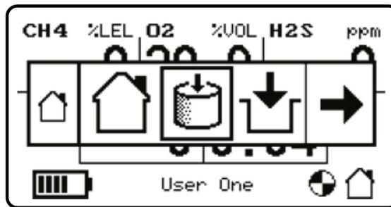
Upon entry to Tank Check Mode, the device will display a confirmation message to inform that alarms are disabled. A single button press will dismiss this screen. The confirmation screen is accompanied by an intermittent warning tone.
