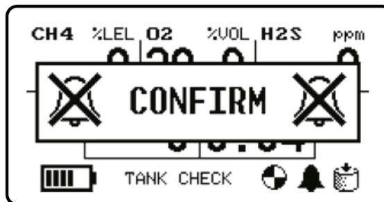
Tank Check Mode can be identified over the Home Screen as the text will be displayed in place of the current user name, the tank check icon will be displayed in the bottom-right corner, and the alarms disabled icon will be displayed to the left of the tank check icon.
