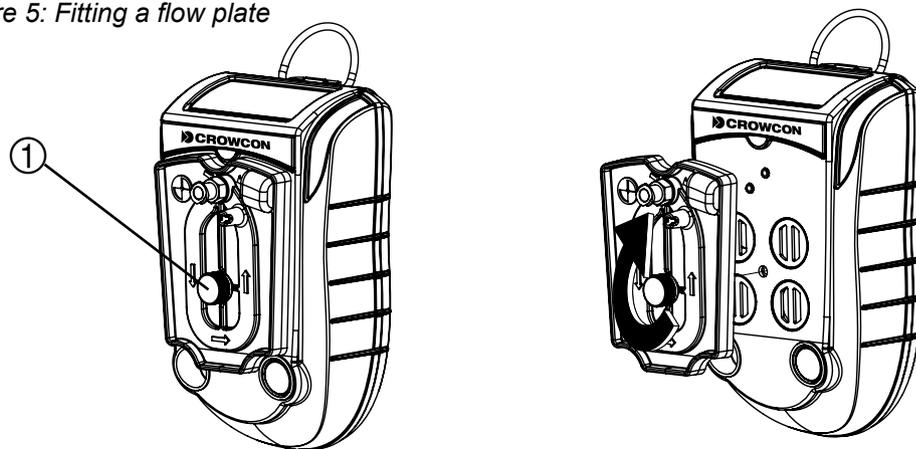
The flow plate includes a quick connect fitting for attaching sample tubes and probes.
