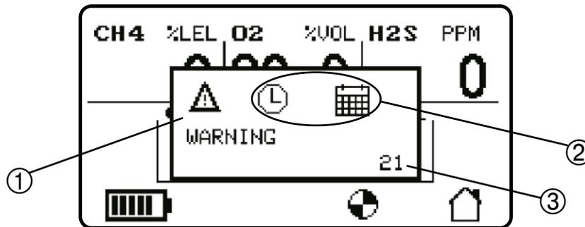
The warning triangle ① indicates faults that can be rectified by the user. The symbol is accompanied by the text “WARNING” below. The warning triangle is replaced by a spanner and screwdriver for faults which require service and the text “SERVICE” below. For the low battery warning the “WARNING” text is replaced by “ALERT”.
