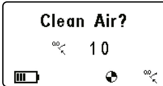
An Autozero should not be performed unless the Gas-Pro is in clean air. Press the operator button to enter the Autozero mode, otherwise the countdown will progress and will not perform a zero.
