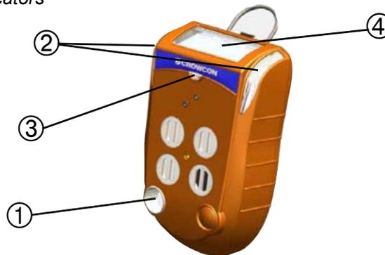
In the alarm state, Gas-Pro will vibrate, its sounder ① will emit a rapid tone, the alarm LEDs ② will flash red and blue, the +ve Safety™ indicator ③ will be off in alarm, the LCD display ④ will also be red and highlight the gas in alarm.
