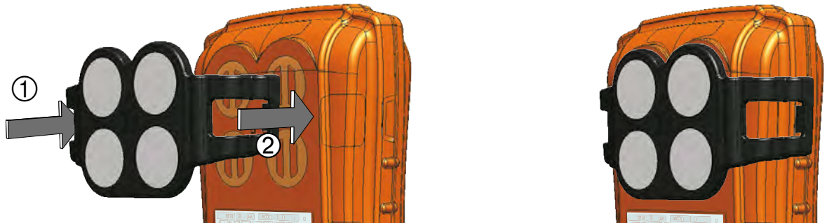
Figure 6: Fitting the external filter plate
