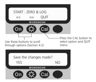
Press the first button to save the change and move the menu back up a level, and the last key to leave the selection as it was (unchanged) and move back up a level.
