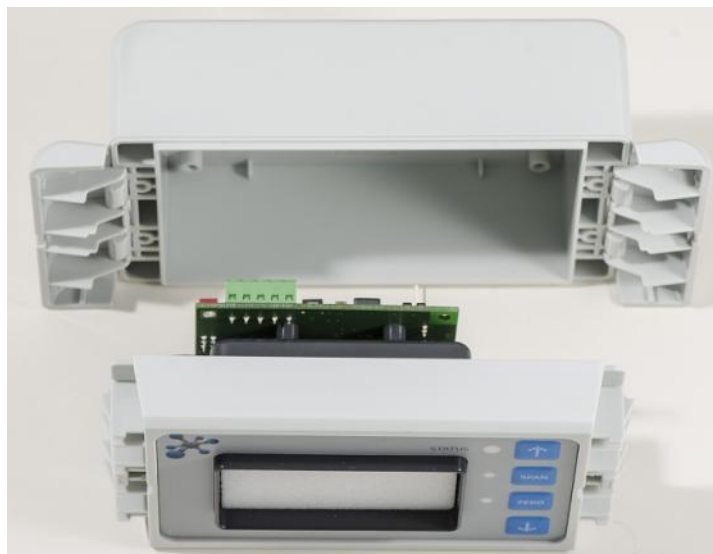
Figure 6: front casing removed
