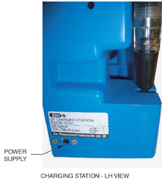
Figure 63: Power Supply to Charging Station
