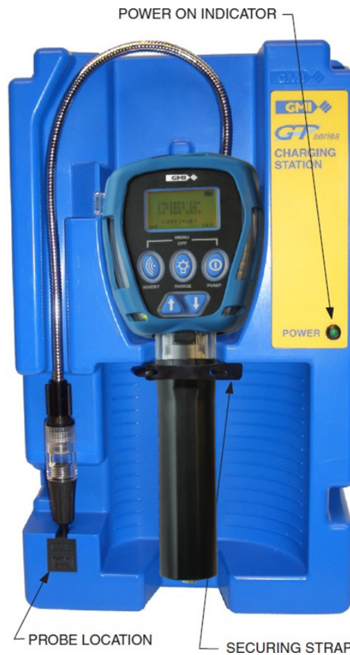
Figure 60: GT Series Charging Station
