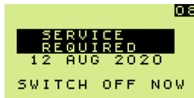
Figure 13: Service Due - Switch Off
