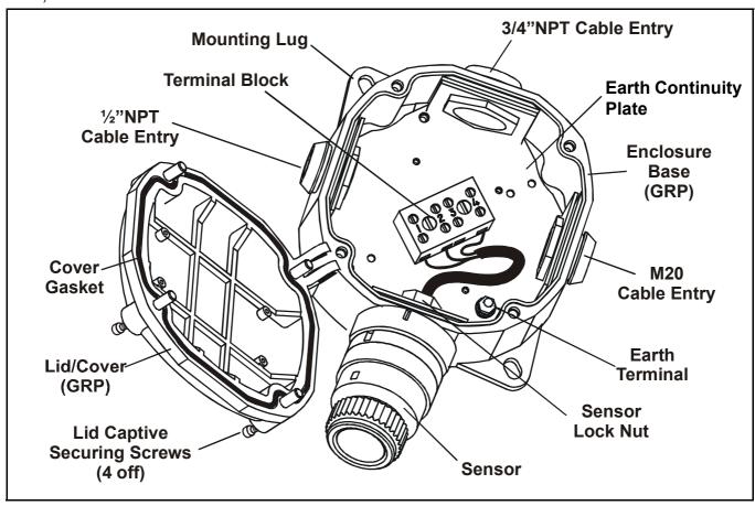
The detector is supplied with one of 3 types of sensor to monitor different gases present in ambient air:
