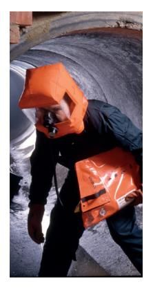
The 3M<sup>™</sup> Scott<sup>™</sup> ELSA (Emergency Life Support Apparatus) is designed for rapid escape from hazardous industrial and marine environments.
