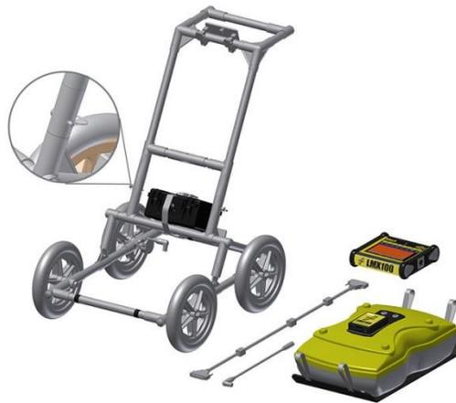
Attach the GPR Sensor to the Cart using the Sensor Support Straps. Ensure the Sensor is oriented the correct way with the connections toward the back of the Cart. Using the Sensor Support Straps, adjust the height of the Sensor so it is 1-2 cm ( $\frac{1}{2}$  –  $\frac{3}{4}$  inch) above the ground. The best way to get a uniform Sensor height is to place a couple of sheets of thick cardboard, particle board or Styrofoam under the sensor before securing the Sensor Support Straps.
