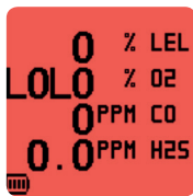
Red display in alarm conditions
