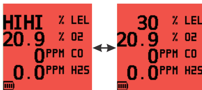
Figure 26: LEL HIHI Alarm
