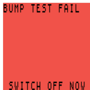
Figure 48: Bump Test Fail - Switch Monitor OFF
