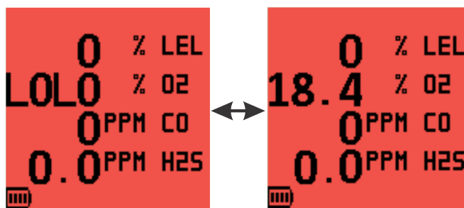
Figure 25: O 2 LOLO Alarm
