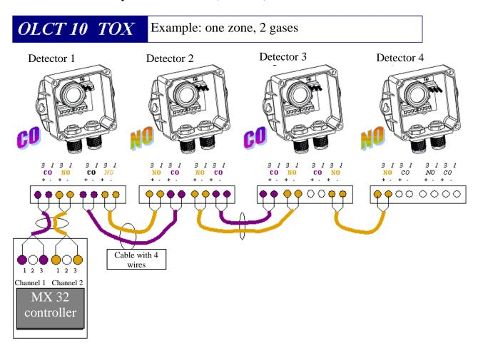
Controller with 2 channels at minimum
