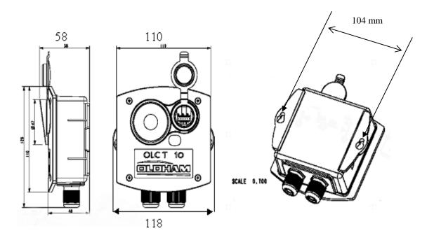
The OLC/OLCT 10 gas detectors-transmitters are mounted vertically with the cable entries positioned downwards.
