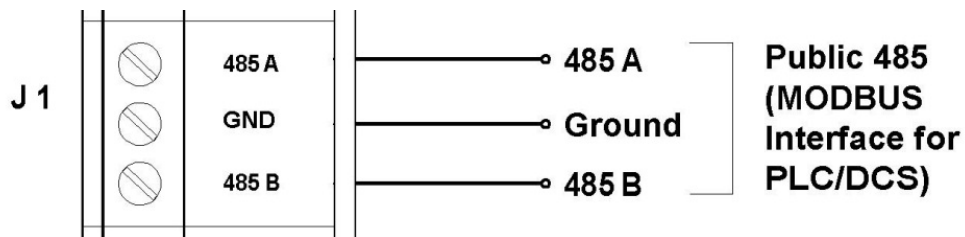
Figure 4-9 Wiring Diagram for the ModBus Interface
