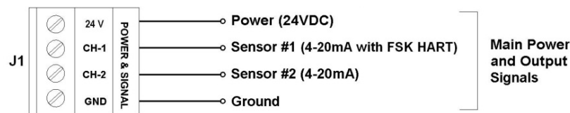
Figure A - 6 Power and Signal Connector J1 on HART Supported iTRANS-2
