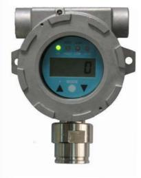
range of toxic gases. It is a flexible detector which provides both an analog (4-20mA) and digital (RS-485, ModBus RTU) output signal. The RAEGuard S uses a smart sensor which can be off-line pre-calibrated. An explosion-proof stainless steel enclosure and magnetic key non-intrusive operation make the RAEGuard S ideal for use in hazardous environments. The RAEGuard S is equipped with a local digital display and LEDs for viewing of gas concentration and alarm conditions.
