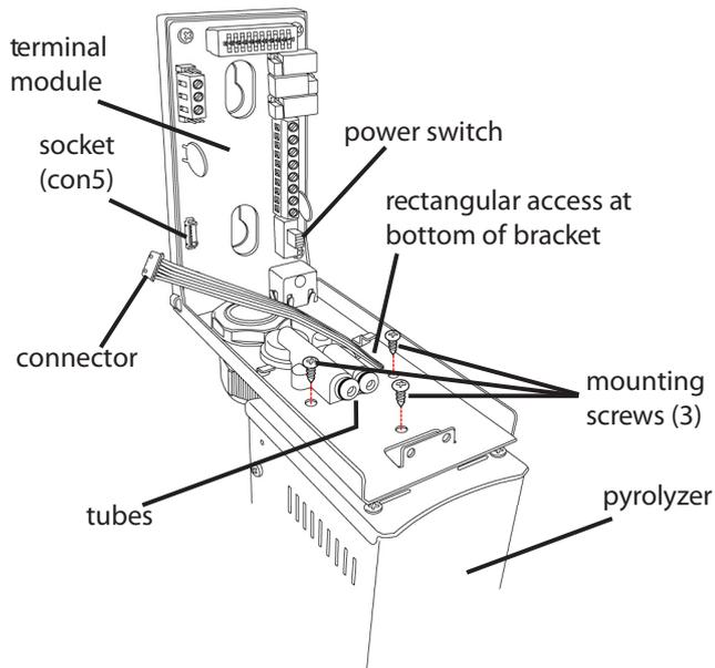
**⚠ WARNING** To maintain sensor accuracy when using the pyrolyzer, do not allow the ambient temperature at the point of installation to exceed 30°C (86°F). Operation above this temperature may require more frequent bump testing or calibration to confirm working specification. Because of the higher operating temperatures when using the pyrolyzer module, Honeywell Analytics strongly recommends that the ventilated Midas Top Cover (shown in Diagram 9-1) be used in all pyrolyzer applications.
