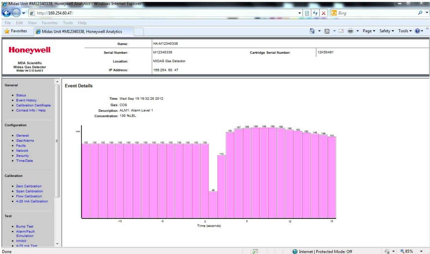
This web page is accessed from the “Details” button from the Event History page. The gas concentration levels for a given alarm are displayed for a period of 30 seconds - 15 seconds before and 15 seconds after the alarm occurred.
