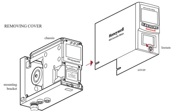
Diagram 8-2. Removing sensor cartridge
