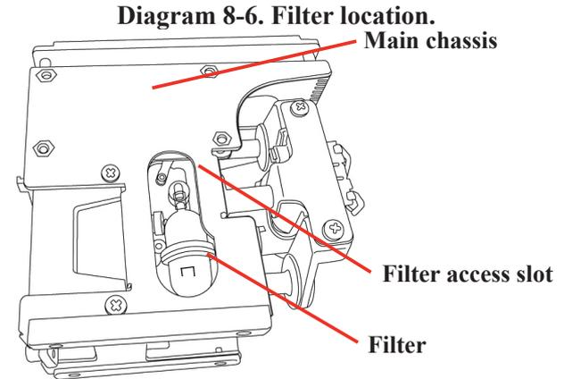
7. Carefully disconnect both sides of the filter from the pump manifold.
