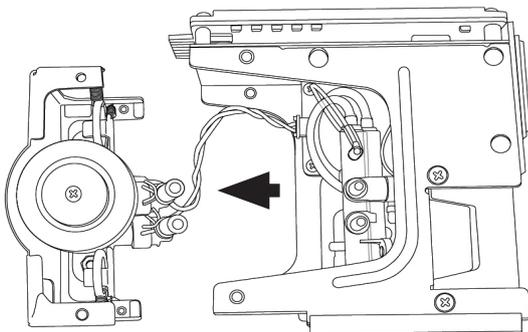
9. Fit the new pump module following the steps above in reverse order. Orient the metal retaining clamps away from the pump wiring to prevent damage. Route pump wiring away from the chassis and manifold to prevent damage.
