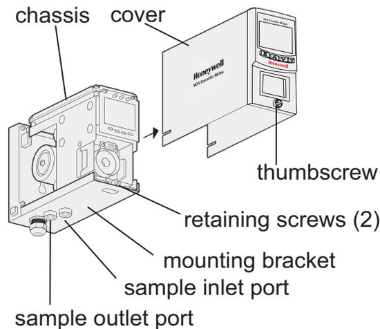
4. Unscrew the two retaining screws located at the bottom front of the chassis.
