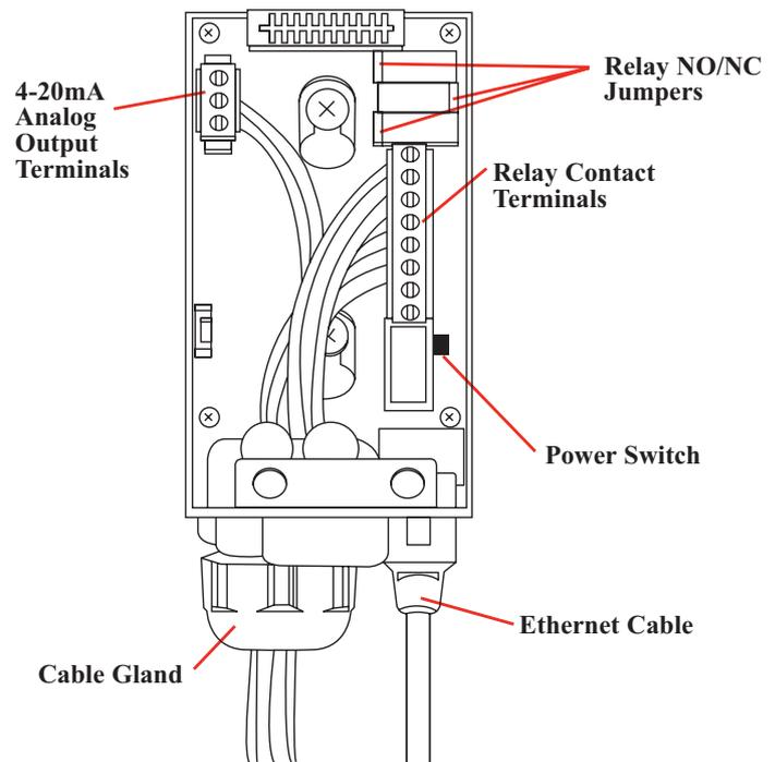
The terminals used are suitable for conductors of 24 to 14 AWG (0.5 to 1.8mm Dia.). The use of 16 AWG (1.5 mm Dia.) conductors is recommended.
