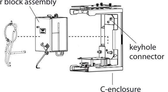
9. Reverse steps 1 through 8 to install the new heater block assembly.
