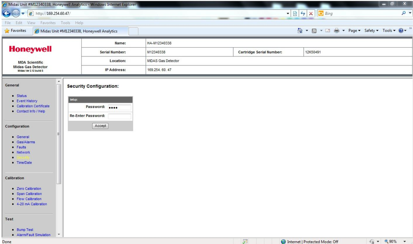
A 4 digit numerical code can be entered to prevent unauthorized changes to the Midas® transmitter; this code can also be entered or changed via the keypad directly on the transmitter. Once activated, each time the user attempts to access a restricted area of the Midas® menu (either directly via the LCD/keypad or via the webpage) they will be prompted to enter the supervisor code.
