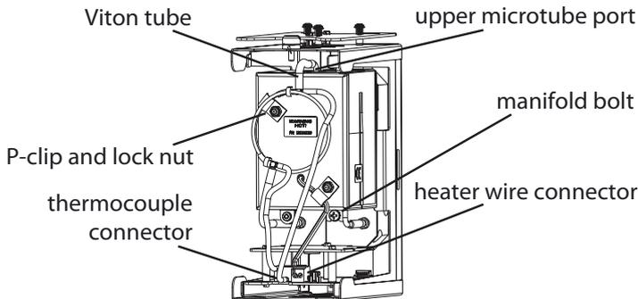
7. Disconnect the lower Viton tube from the quartz tube port. (If necessary, swing the heater unit as shown in Diagram 9-13.) Discard the old Viton tube.
