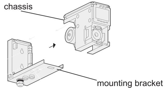
6. Thread the connector and wire harness from the pyrolyzer through the rectangular access in the bottom of the mounting bracket.
