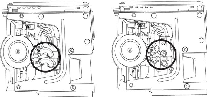
8. Slide the pump module out and disconnect the connector from the pcb.
