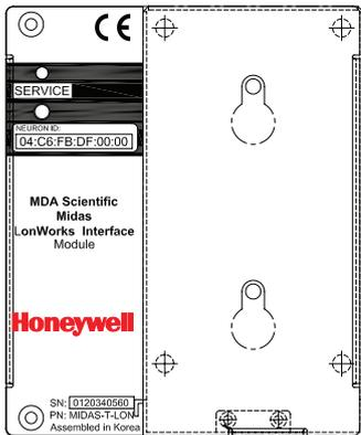
The Midas® uses the Free Topology (FT) physical layer which communicates at 78 Kbaud. Each FT segment can contain up to 64 nodes and up to 2.7 Km of cable. Routers permit expansion of the network to multiple segments.
