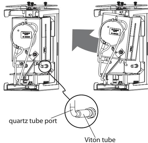
8. Remove the heater block assembly by first lifting it up and then sliding it out of the keyhole connector in the C-enclosure (Diagram 9-14).
