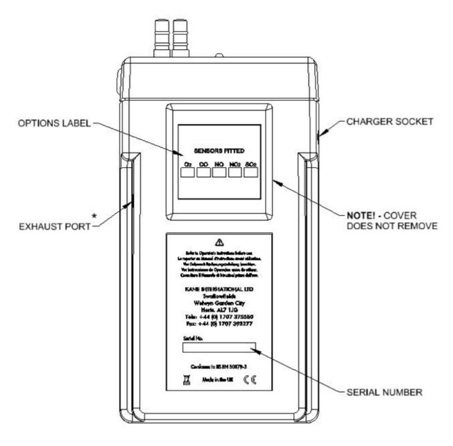
**NOTE:** Do NOT cover exhaust port as this will severely affect analyser operation
