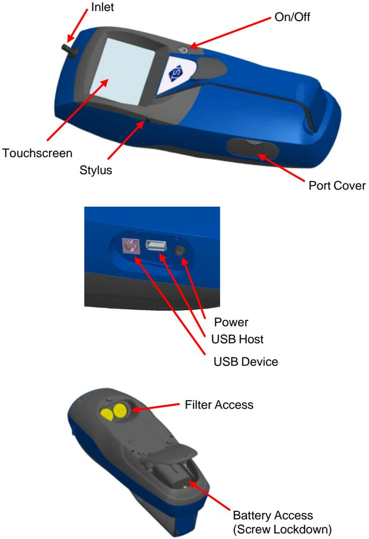
**Figure 1-3: Features on Handheld Model**
