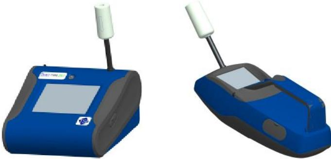
**Figure 4-1: Attach Zero Filter to Inlet**
