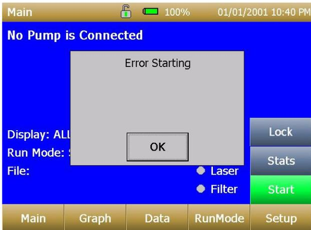
3. If the pump **IS NOT** connected while attempting to perform a Zero Cal, an error appears on the Setup screen.
