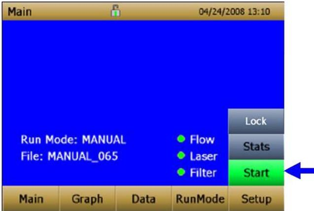
When the instrument is on, but not taking any mass measurements the start button will be green and instruments pump will not be running. To start taking a measurement, press the green **Start** button.
