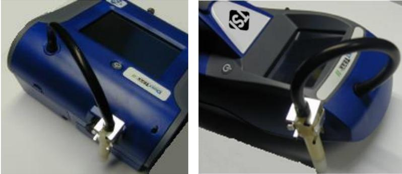
**Figure 2-8: Installing Door-Oliver Cyclone**
