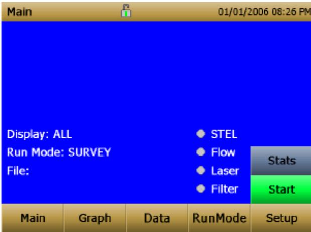
Use a stylus or fingertip, touch the “buttons” on the screen to activate different menus.
