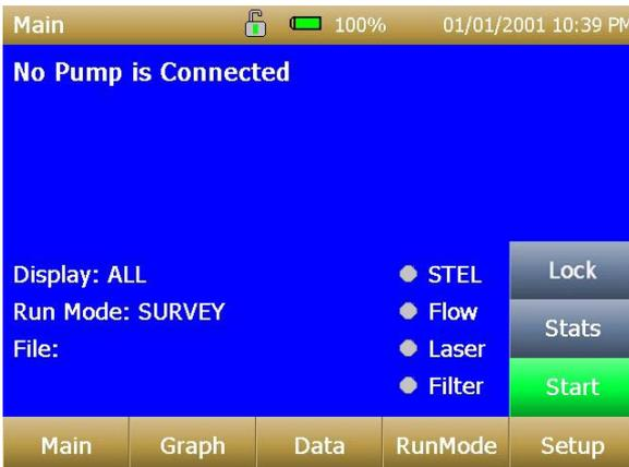
Connect the External Pump Module to the DustTrak™ monitor and then try again. TSI® recommends powering down the DustTrak™ monitor before connecting the External Pump Module to the DustTrak™ monitor. Connect the power cable and the flow tubing between the DustTrak monitor and the External pump module, as applicable.
