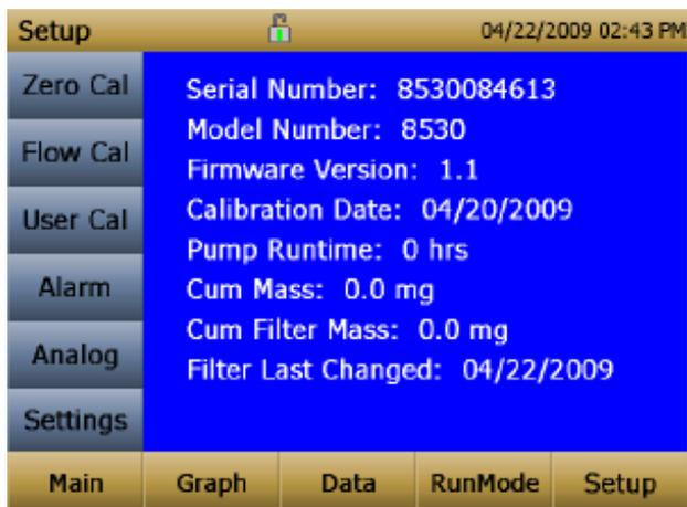
Pressing **Setup** activates the Setup Menu touchscreen buttons along the left edge of the screen. Setup is not accessible when the instrument is sampling.
