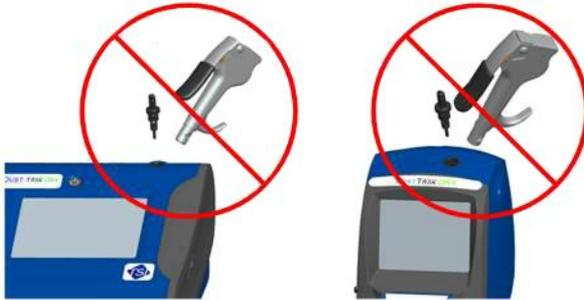
Figure 4-3: DO NOT Blow into Instrument
