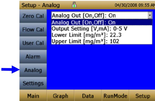
**Analog** setup screen sets the parameters that will drive the analog out port. Applies to the 8530 Desktop model only.
