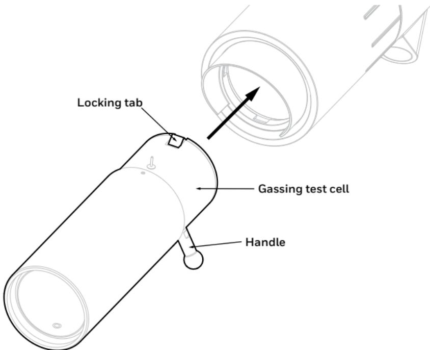
2. Rotate the handle clockwise to lock the gassing test cell onto the receiver.
