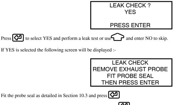
Once the test has PASSED remove the probe seal and press
