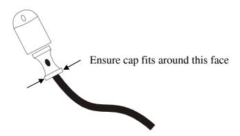
Press when the seal is in place. The check will take a few seconds. Following a successful test the analyser will return to the **MAIN DISPLAY**.
