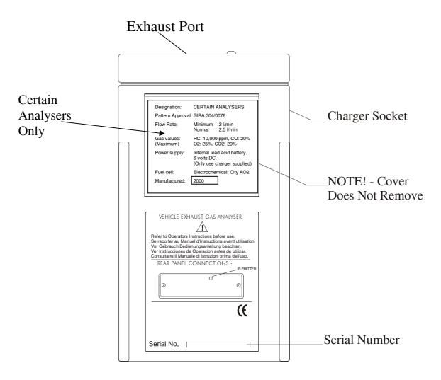
\*NOTE! Do not cover exhaust port as this will severely affect analyser operation
