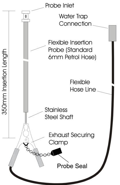
**Note:** A variety of probes are available, including high temperature probes necessary for on-road / rolling road vehicle testing when the temperature of the emission gases increase. Please request further details from your distributor or contact Kane International Ltd directly.
