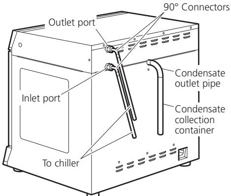
Optimum performance will be obtained with the connection tubing as short as possible. Observe the specification of the chiller for acceptable tubing lengths and maximum head height. Place the chiller in a position which is safe in order to prevent accidental collision.
