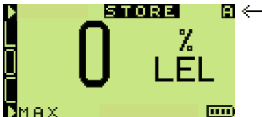
Fig. 3-34 Alarm Enabled Identifier
