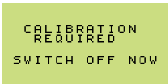
Fig. 4-12 Calibration / Configuration Memory Fault
