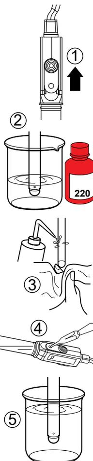
1. If the pH electrode is liquid-filled, uncover the refilling port.
