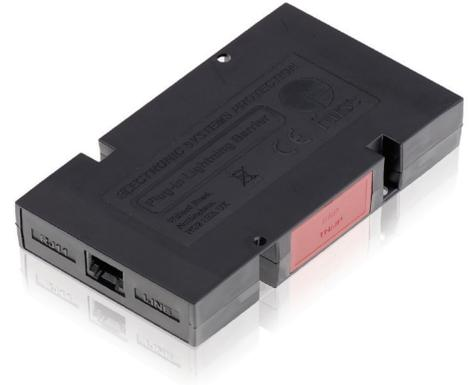
Combined Category D, C, B tested protector (to BS EN 61643) suitable to protect telephony equipment plugged into a BT telephone (BS 6312), Modem (RJ11) or ISDN (RJ45) socket. For use at boundaries up to LPZ 0 to protect against flashover (typically the service entrance location) through to LPZ 3 to protect sensitive electronic equipment.
