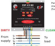
Parallel connection to three phase star (4 wire and earth) supplies (fuses not shown for clarity)
