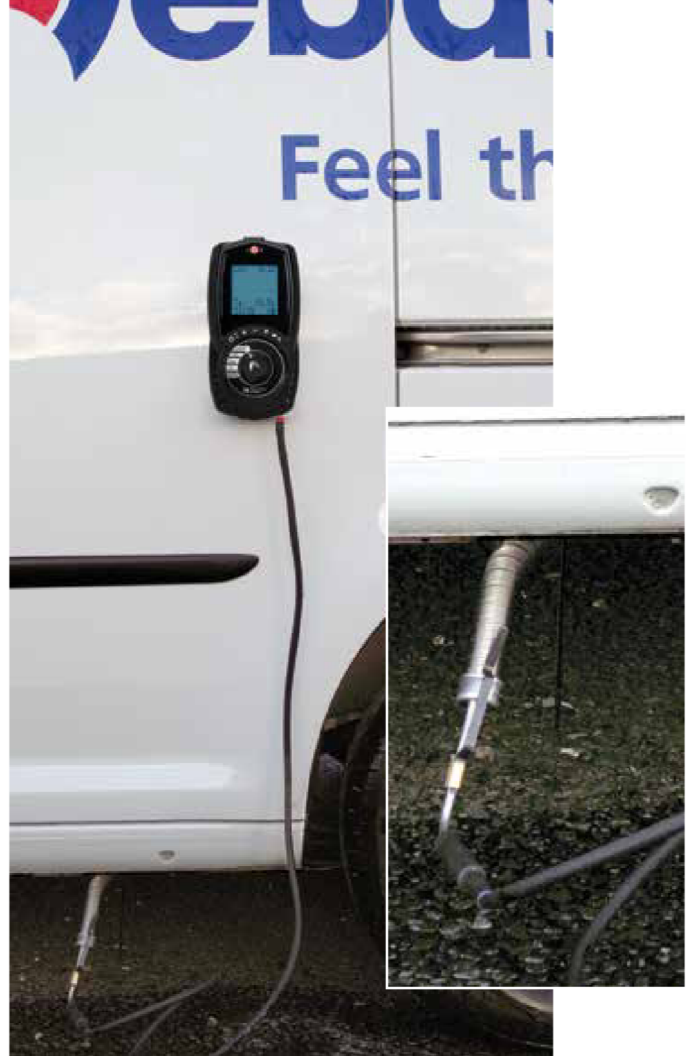
Auxiliary Heater CO 2 measurement
