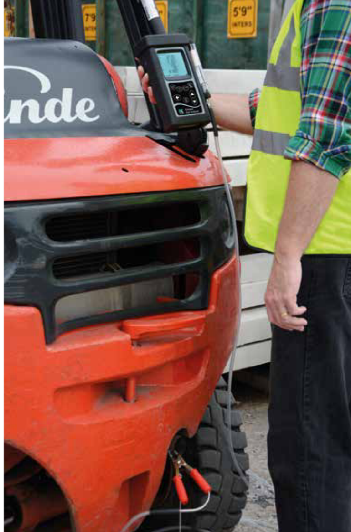
Fork lift truck exhaust emissions measurement
